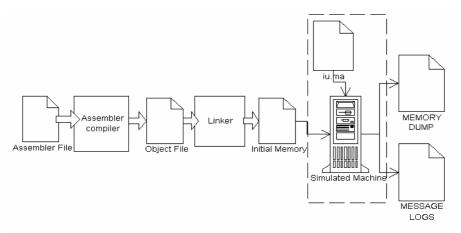
Fig. 18. Process of simulation from the assembler file to the memory dump.
