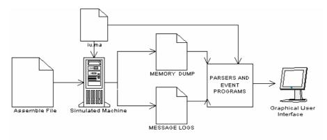
Fig. 24. Dynamic process used to generate a GUI.
