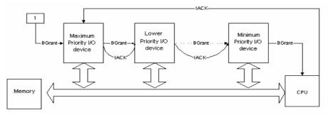
Fig. 6. Active components BGRANT chain [Wainer et al. 2002].
