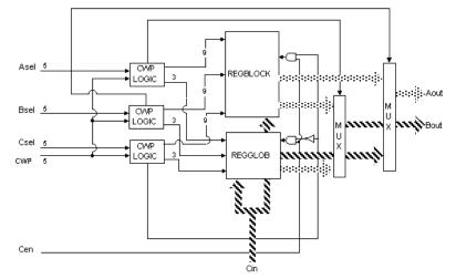
Figure 2. Organization of the processor's registers.
