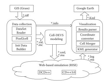
*Figure* 17.7 Web-based simulation architecture using Cell-DEVS and geographic information system.
