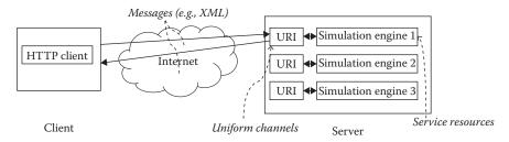
Figure 17.6 Distributed simulation RESTful Web service architecture.
