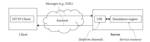
Figure 17.3 Basic remote simulation architecture with RESTful Web service.
