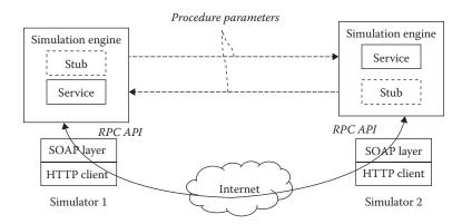
Figure 17.5 Distributed simulation SOAP-based Web service architecture.
