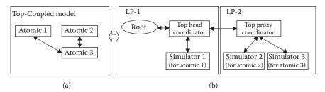
*Figure* 17.15 Head/Proxy Modeling Structure. (a) Coupled model defined. (b) Model hierarchy during simulation. (Al-Zoubi, K. and Wainer, G., Performing distributed simulation with RESTful Web-services, *Proceedings of the 2009 Winter Simulation Conference*, Austin, TX, © 2009 IEEE.)
