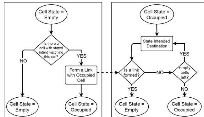
Figure 6 State Diagram for movement [15]
