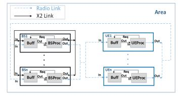
Fig. 2. Simplified DEVS model for CoMP control architecture
