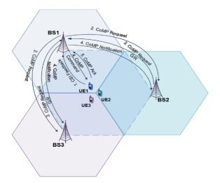
Fig. 1. Message transfer to elect CS and establish CoMP in DCEC-HetNet
