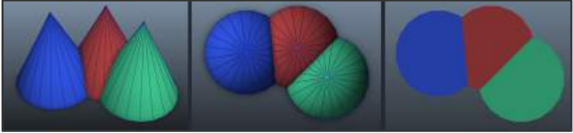
Figure 3.8 The PSM is implemented as a 2D bitmap composed of truncated Voronoi cells created by a top-view orthogonal projection of 3D cones; underneath an obstacles overlay.
