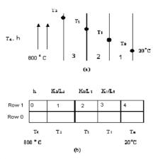
Figure 2. (a) Steady-state heat transfer through a composite wall. (b) The problem as a Cell-DEVS space.
