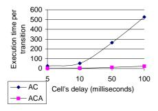
Figure 9. Simulation execution times of Cell-DEVS models
