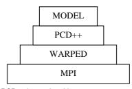
Figure 3. PCD++ layered architecture
