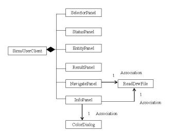
Figure 18. Class diagram of the visualization applet.
