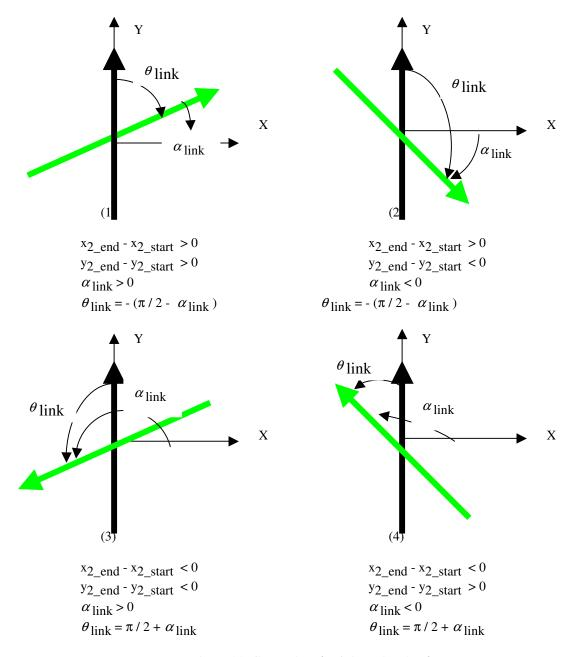
Figure 20. Computing the Orientation Angle
