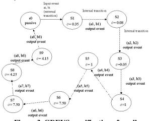
**Figure 3. GDEVS specification of a cell.** Using the polynomial definitions in Table 1, we can now define the behavior of each of the cell's local computing functions, which is described by the GDEVS state graph in the figure
