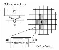
Fig. 2. Description of a Cell-DEVS atomic model.
