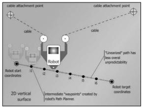
Figure 1: Robot path between start and target coordinates using a path planner
