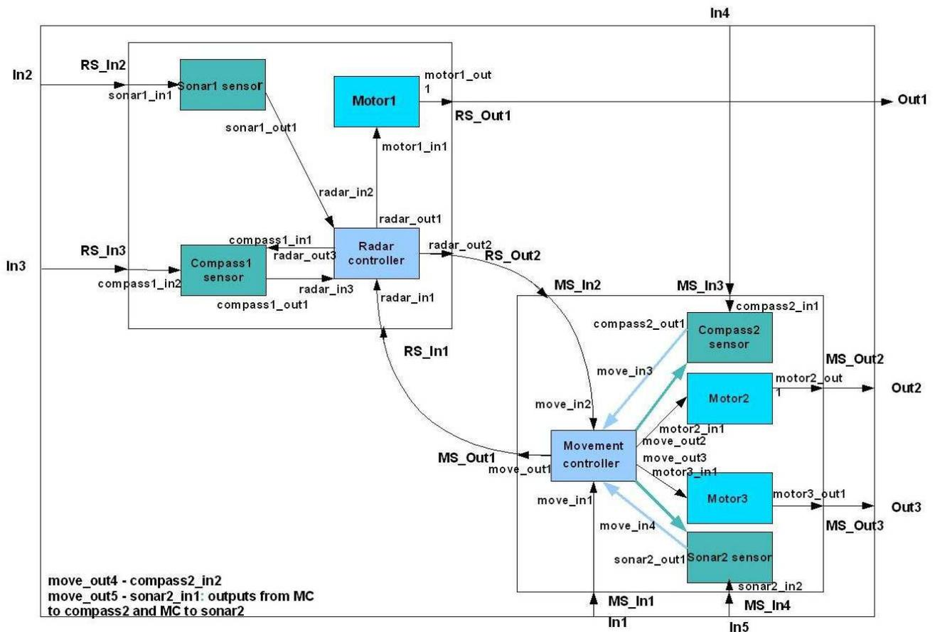
Figure 3. Detective robot DEVS model hierarchy
