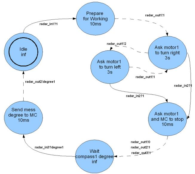
Figure 4. *Radar controller* GGAD diagram
