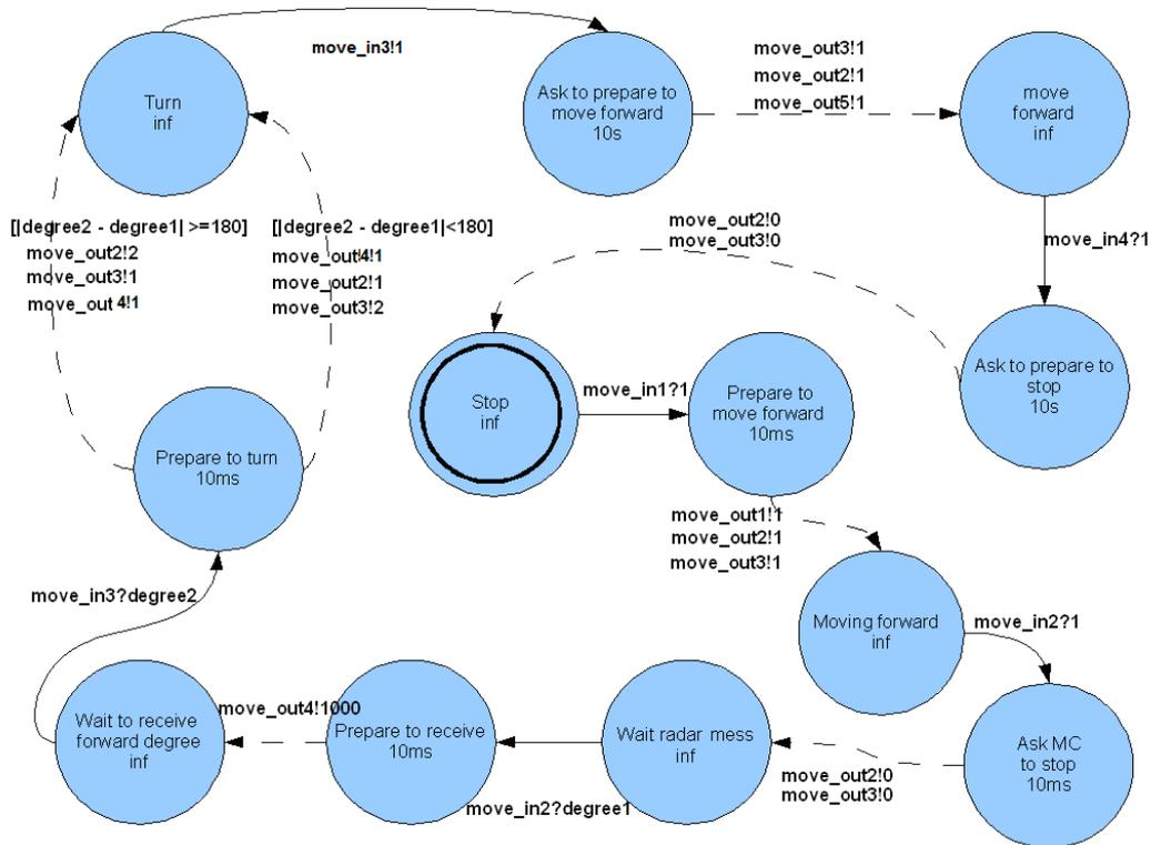
Figure 5. GGAD state diagram of Movement controller
