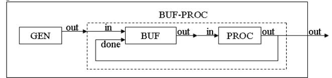
**Figure 1.** Generator-Buffer-Processor hierarchical DEVS model
