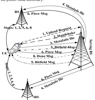
Figure 3. Segmented Upload Algorithm Message Transfer
