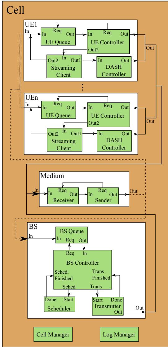
Fig. 3. Coupled DEVS model of DABAST.
