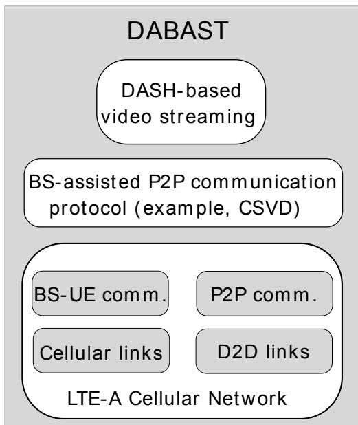
Fig. 1. The DABAST architecture.
